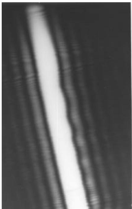
Figure 2. Experimental results with the arrangement of figure 1. The direction of light- and shadow-side is fixed by the half-plane. Enlargement of a negative at which the exposure-time was fitted to the higher orders.
