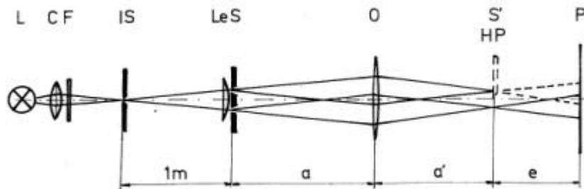
Figure 3. Experimental arrangement for double-slit with intermediate imagery with indicated optical path. L - light-source, a super-pressure mercury-lamp HBO 100; C - condenser; F - green-filter; IS -illumination slit; Le - lens  $f' = 1\text{ m}$ ; S - double-slit; O - telescope-objective  $f' = 60\text{ cm}$ , diameter  $10\text{ cm}$ , a best-form lens; S' - the image of the double-slit, HP - half-plane, a razor-blade on a carriage with a micrometer-screw; P - photographic film.
