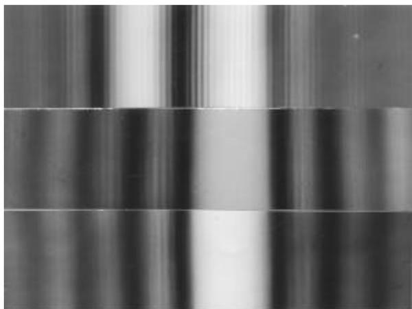
Figure 4. Experimental results of masking one image of the double-slit in the arrangement figure 3. With  $-a = a' = 1.2\text{ m}$ ,  $e = 1\text{ m}$ , IS -  $0.15\text{ mm}$ , S - single slit-width  $0.25\text{ mm}$  and  $1.5\text{ mm}$  intermediate piece.
