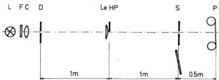
Figure 1. Experimental arrangement for diffraction following one after another. L - light-source, a super-pressure mercury-lamp HBO 100; F - green-filter; C - condenser; D - pinhole-diaphragm, a spinning nozzle 50  $\mu$ m; Le. - lens  $f' = 1$  m; HP - half-plane, a razor-blade; S - slit 0.3 mm,  $10^\circ$  towards HP oblique; P - photo-film in a miniature-camera without optic.
