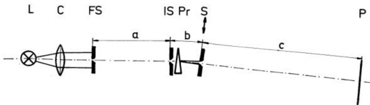
Figure 1. Experimental arrangement for coloured inhomogeneous illumination. L - light-source, a high-pressure mercury lamp; C - condenser; FS - first illumination-slit; IS - second illumination-slit 0.15 ... 0.3 mm; Pr - prism, crown glass 10°...30°; S - diffraction-slit 0.3 mm; F - incident plane, a photo-plate. a = 1 m, b = 120...400 mm, c = 0.25...4 m
